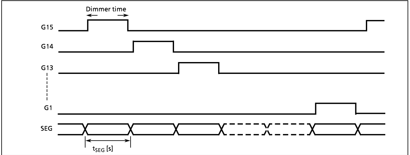
Figure 2-58. VFT Drive Waveform (with 9 Segments and 15 Digits)
