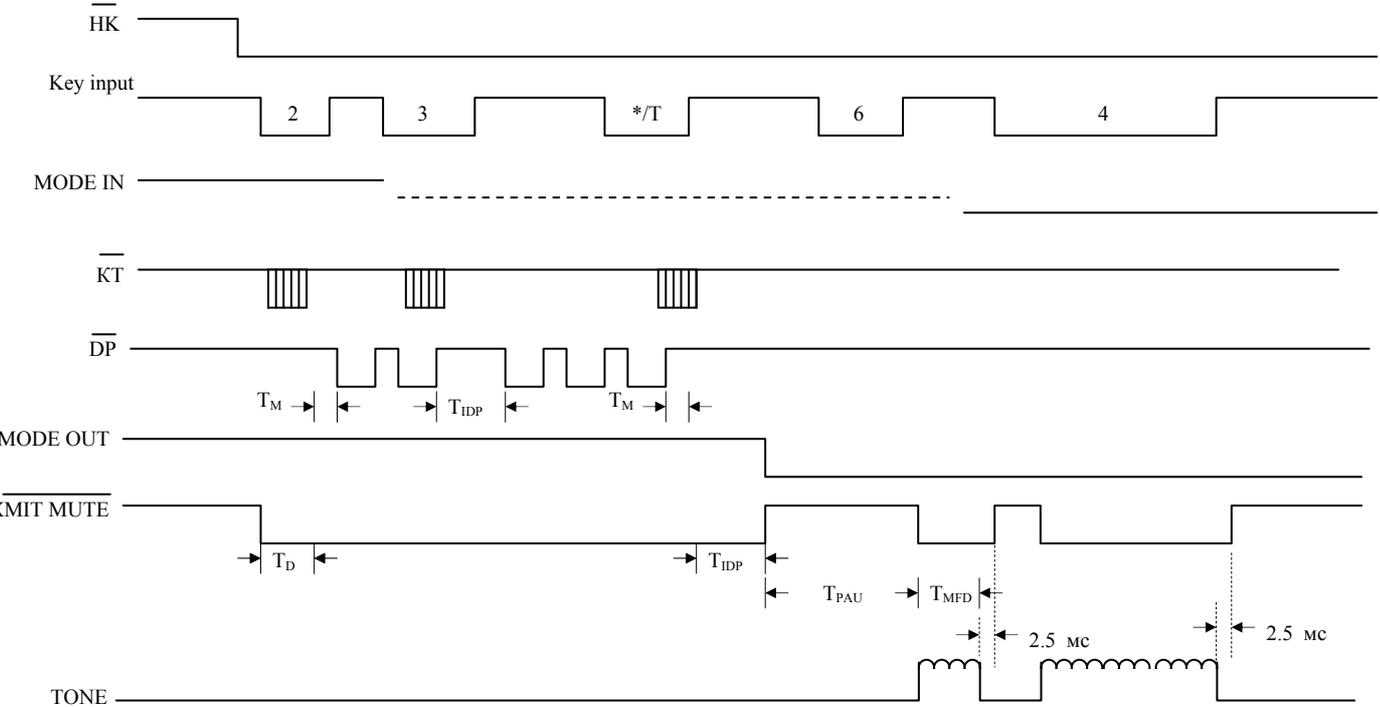
6. One key redial using RD key (DTMF mode for example).
