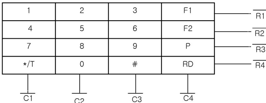
1. \*/T – At Pulse mode this key works as Pulse -> DTMF key (T key), at DTMF mode the key works as \*key. \*/T key will occupy one memory digit in either use.
