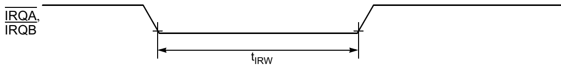
Figure 10-6 External Interrupt Timing (Negative Edge-Sensitive)
