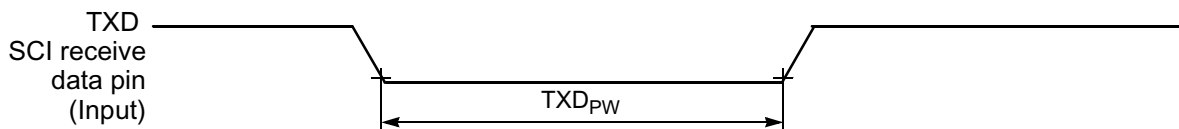
Figure 10-17 TXD Pulse Width
