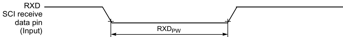
Figure 10-16 RXD Pulse Width
