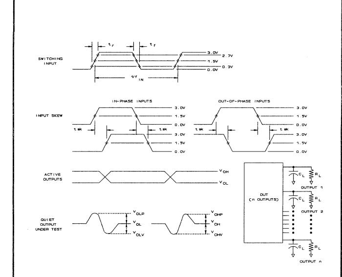
$C_1$  = 47 pF -0 percent, +20 percent chip capacitor plus  $\ge$  3 pF of equivalent capacitance from the test jig and probe.
