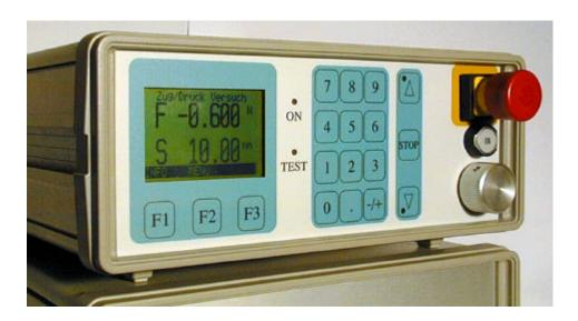
EDC100 on top of a DDA04 (500W) /05 (1000W) power amplifier. All electronics you need for a e.g. up to 100 kN testing instrument
