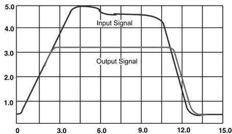
FIGURE 1. Typical NMOS Bus Switch Waveform
