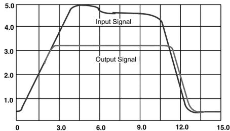
FIGURE 1. Typical NMOS Bus Switch Waveform
