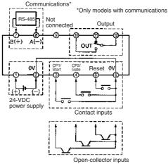
Note: (2) and (6) are connected internally.
