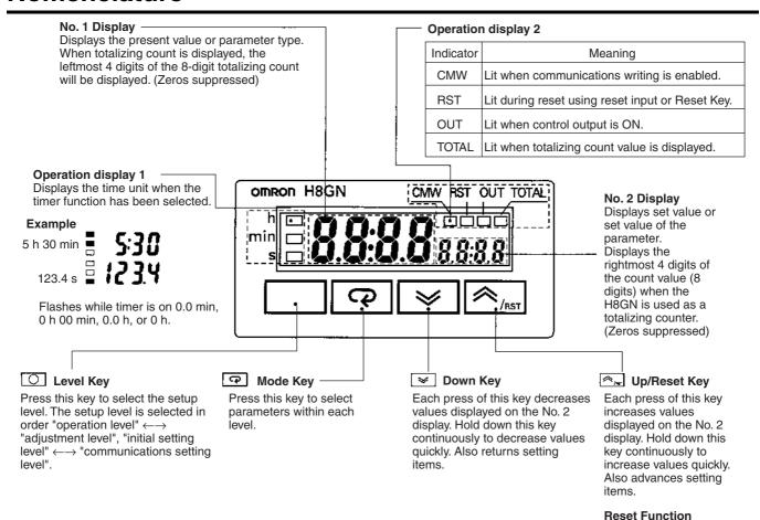
To reset the present value, press this key while the present value is displayed. If this key is pressed while the totalizing count value is displayed, the totalizing count value and the present value will be reset.
