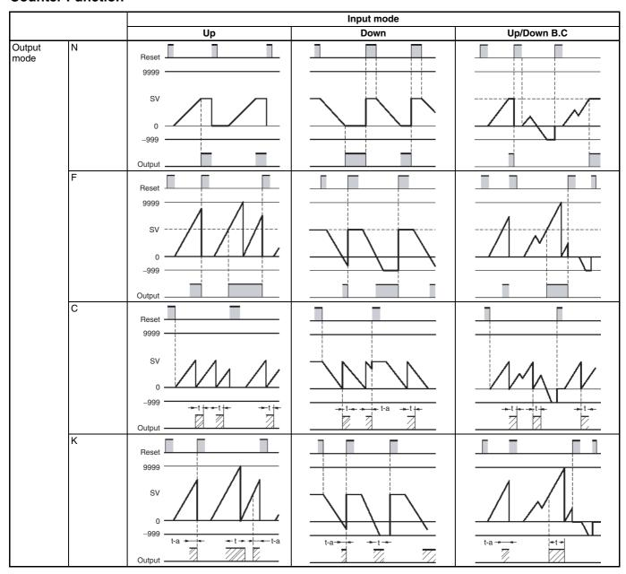
Note: 1. t: output time. t - a < t: Less than the output time.
