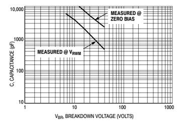
Figure 3. Capacitance versus Breakdown Voltage
