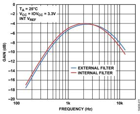
Figure 12. Input Filter Frequency Response
