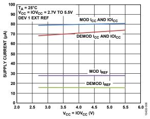
Figure 8. Supply Currents vs. Supply Voltage—External Reference
