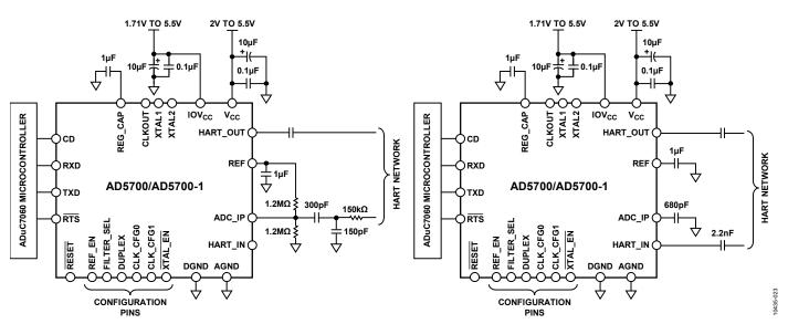
Figure 26. AD5700/AD5700-1 Typical Connection Diagram for External and Internal Filter Options
