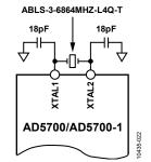
Figure 23. Crystal Oscillator Connection
