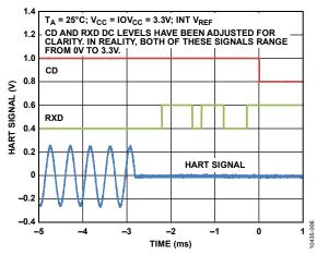
Figure 6. Carrier Detect Off Timing
