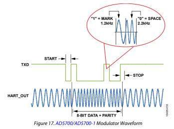
The modulator block contains a DDS engine that produces a 1.2 kHz or 2.2 kHz sine wave in digital form and then performs a digital-to-analog conversion. This DDS engine inherently generates continuous phase signals, thus avoiding any output discontinuity when switching between frequencies. For more information on DDS fundamentals, see MT-085, *Fundamentals of Direct Digital Synthesizers (DDS)*. Figure 18 demonstrates a simple implementation of this FSK encoding.
