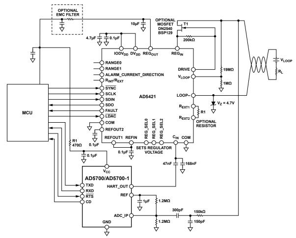
Figure 27. Loop-Powered Transmitter Diagram
