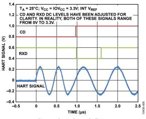
Figure 5. Carrier Detect On Timing
