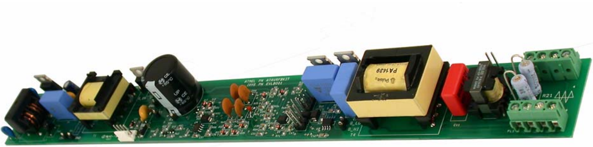
Figure 1-2. Ballast Demonstrator Board
