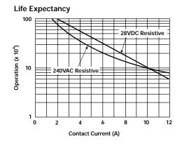
**Note:** This data is based on the max. allowable temperature for E type insulation coil (115°C).
