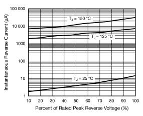
Fig. 5 - Typical Reverse Leakage Characteristics
