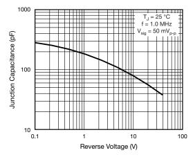
Fig. 6 - Typical Junction Capacitance
