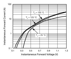
Fig. 4 - Typical Instantaneous Forward Characteristics
