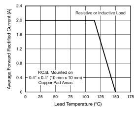
Fig. 1 - Forward Current Derating Curve
