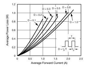
Fig. 2 - Forward Power Loss Characteristics
