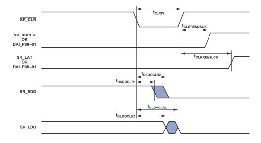
Figure 45. Shift Register Reset Timing
