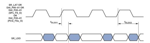
THE TIMING PARAMETERS SHOWN FOR  $t_{DLDO1}$  AND  $t_{DLDO2}$  ARE ALSO VALID FOR  $t_{DLDODAI1}$ ,  $t_{DLDODAI2}$ ,  $t_{DLDOPCG2}$ ,  $t_{DLDOPCG3}$ , AND  $t_{DLDOPCG2}$ .
