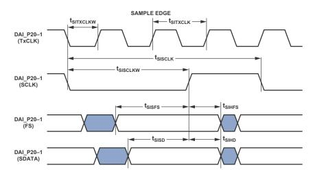
Figure 34. S/PDIF Transmitter Input Timing
