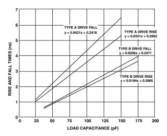
Figure 50. Typical Output Rise/Fall Time (20% to 80%,  $V_{DD\ FXT} = Max$ )
