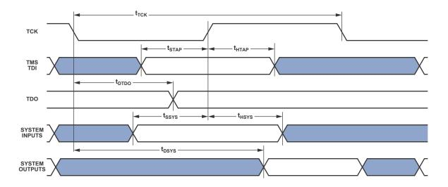
Figure 46. IEEE 1149.1 JTAG Test Access Port
