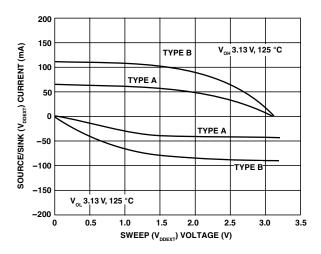
Figure 47. Typical Drive at Junction Temperature
