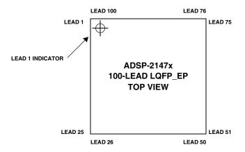
Figure 53. 100-Lead LQFP\_EP Lead Configuration (Top View)
