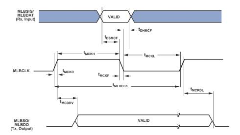
Figure 39. MLB Timing (5-Pin Interface)
