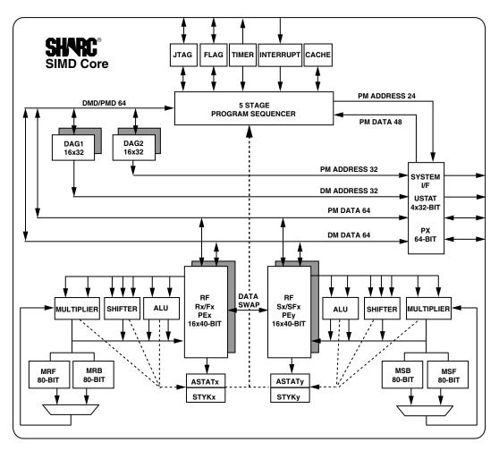
Figure 2. SHARC Core Block Diagram
