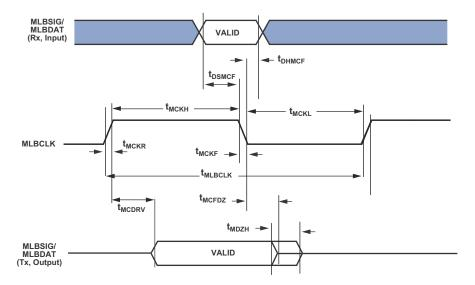
Figure 38. MLB Timing (3-Pin Interface)
