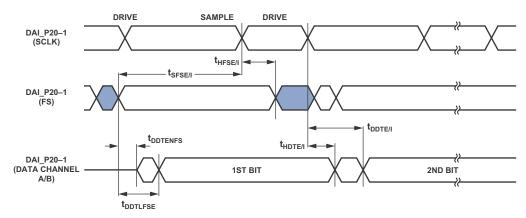
Figure 23. External Late Frame Sync<sup>1</sup>
