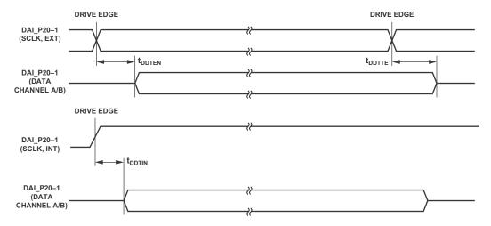
Figure 24. Enable and Three-State
