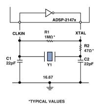
R2 SHOULD BE CHOSEN TO LIMIT CRYSTAL DRIVE POWER. REFER TO CRYSTAL MANUFACTURER'S SPECIFICATIONS
