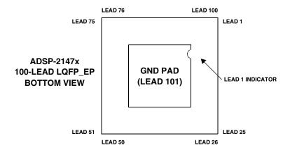
Figure 54. 100-Lead LQFP\_EP Lead Configuration (Bottom View)
