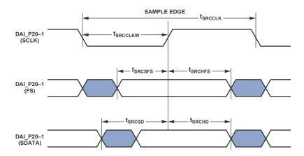
Figure 28. ASRC Serial Input Port Timing
