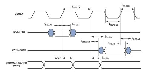
Figure 19. SDRAM Interface Timing
