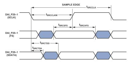
Figure 29. ASRC Serial Output Port Timing
