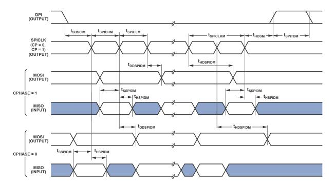
Figure 36. SPI Master Timing
