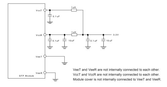
Figure 14. Recommended Supply Filtering Network
