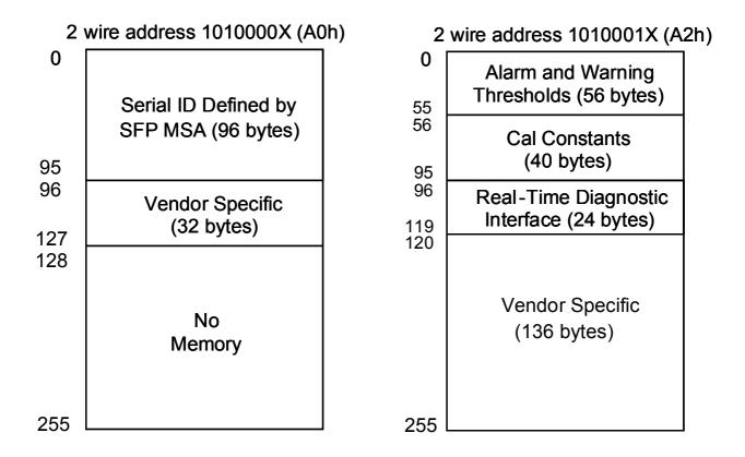
Figure 11. Digital Diagnostic Memory Map (A2h is applicable for SCP6EP4-GL-#N-xx)
