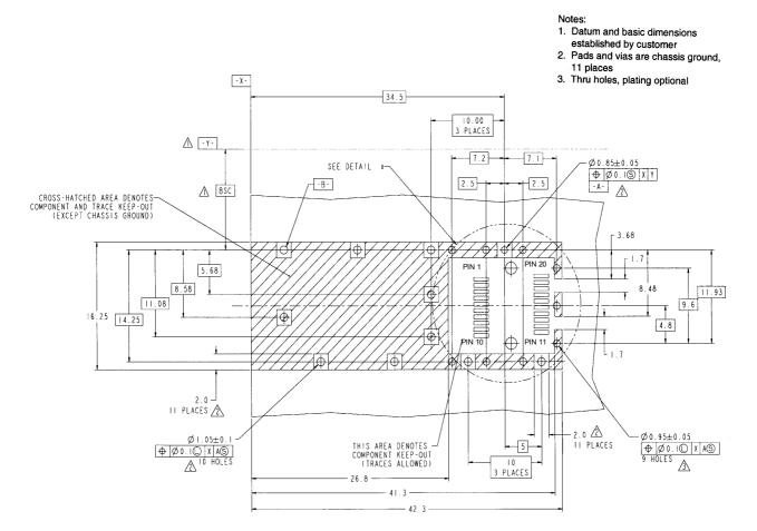
Figure 5. SFP Host Board Mechanical Layout (Cont.)
