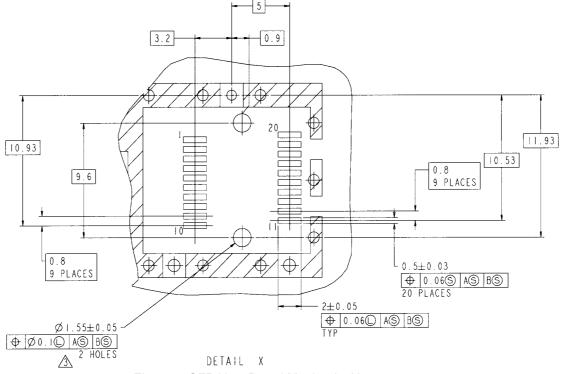
Figure 4. SFP Host Board Mechanical Layout
