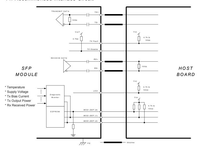
Figure 13. Recommended Interface Circuit (Diagnostic Monitor is incorporated for SCP6EP4-GL-#N-xx only.)
