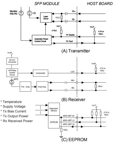
Figure 1. Block Diagram (Diagnostic Monitor is incorporated for SCP6EP4-GL-#N-xx only.)
