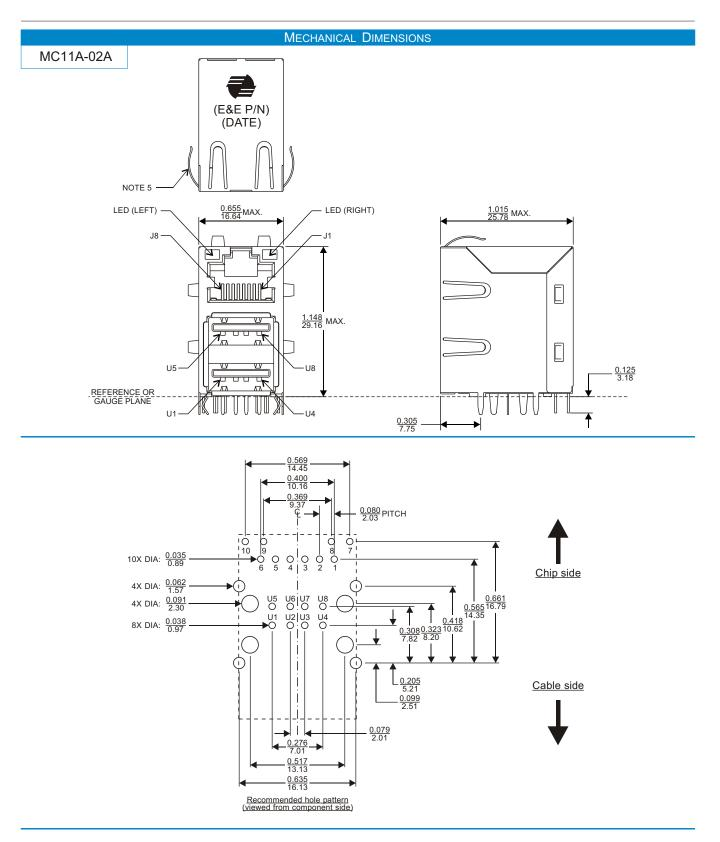
All dimensions are specified in  $\frac{\text{inch}}{\text{mm}}$ with higher precedence in inch. Unless otherwise specified, all tolerances are  $\pm \frac{0.010}{0.25}$
