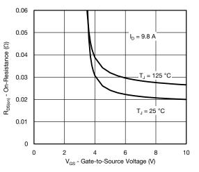
**On-Resistance vs. Gate-to-Source Voltage**
