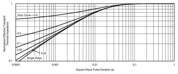
Normalized Thermal Transient Impedance, Junction-to-Case
