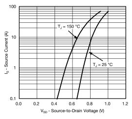
Source-Drain Diode Forward Voltage
