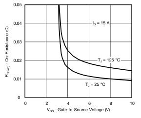
**On-Resistance vs. Gate-to-Source Voltage**
