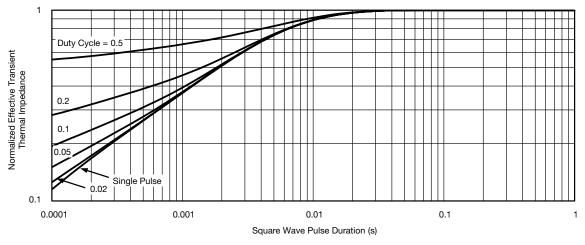
Normalized Thermal Transient Impedance, Junction-to-Case
