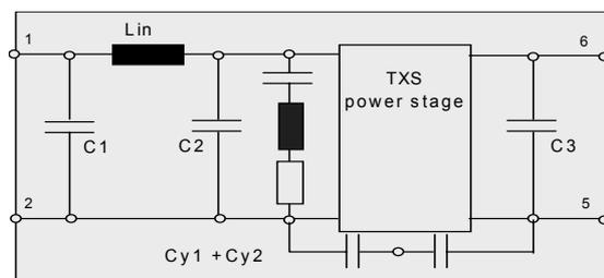
Figure 52: On board input and output filters.
