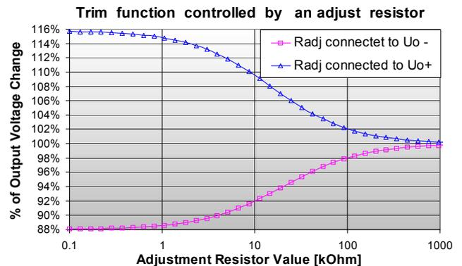
Figure 31: Trim with an external adjust resistor
