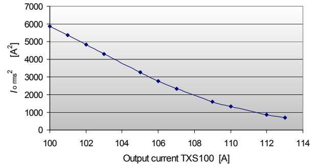
Figure 39: Function of I<sub>o\_rms</sub><sup>2</sup>, proportional to the thermal energy at the overload location
