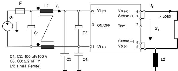
Figure 48: TXS100ZB-N with a one stage input filter according figure 44 and an inductor in the ground line to the output.  $L2 = 9.6 \text{ mH}$ ,  $\mu_1 = 50'000$ , (VAC W620)
