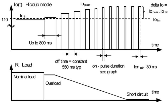
Figure 37: Hiccup Timing at Overload
