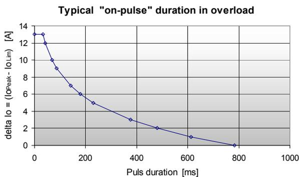
Figure 38: Characteristic of over current protection
