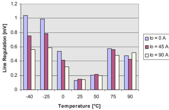
Figure 9: Line Regulation TXS100ZD
