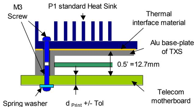
Figure 56: Screw fixing of the TXS converter
