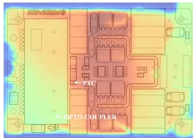
Figure 41: TXS100-ZY at 300 LFM,  $U_i = 48$  V,  $I_o = 100$  A,  $T_A = 27.9$  °C,  $T_{BP} = 59.7$  °C,  $T_{PCBmax} = 74.1$  °C,  $dT = 14.4$  K
