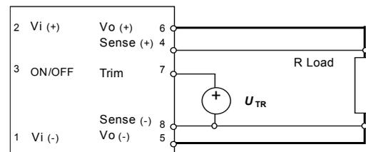
Figure 32: Trim up and down with an external voltage source referenced to sense (-)
