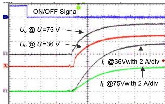
Ch 1:  $I_{in}$  @ 75 V, 2 A/div., Ch R1:  $I_{in}$  @ 36 V, 2 A/div.
