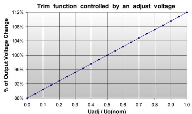
Figure 33: Trim with an external adjust voltage
