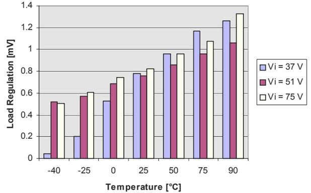
Figure 10: Load Regulation TXS100ZD
