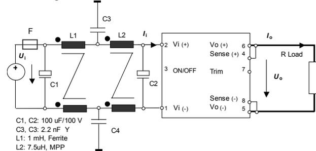
Figure 46: TXS100ZB-N with a two stage input filter:
