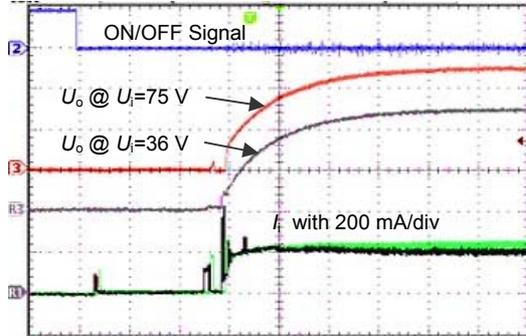
Ch 1:  $I_{in}$  @ 75 V, 0.2 A/div., Ch R1:  $I_{in}$  @ 36 V, 0.2 A/div.
