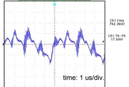
Figure 17: Output Ripple TXS100ZD
