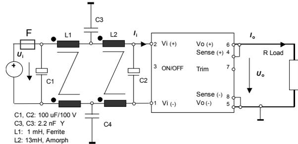
Figure 50: TXS100ZB-N with a two stage input filter and ground output.
