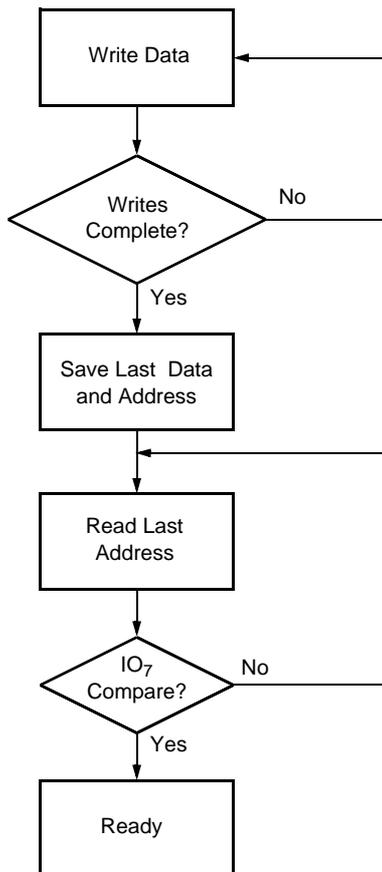
$\overline{DATA}$  Polling can effectively reduce the time for writing to the X28HC64. The timing diagram in Figure 2 illustrates the sequence of events on the bus. The software flow diagram in Figure 3 illustrates one method of implementing the routine.
