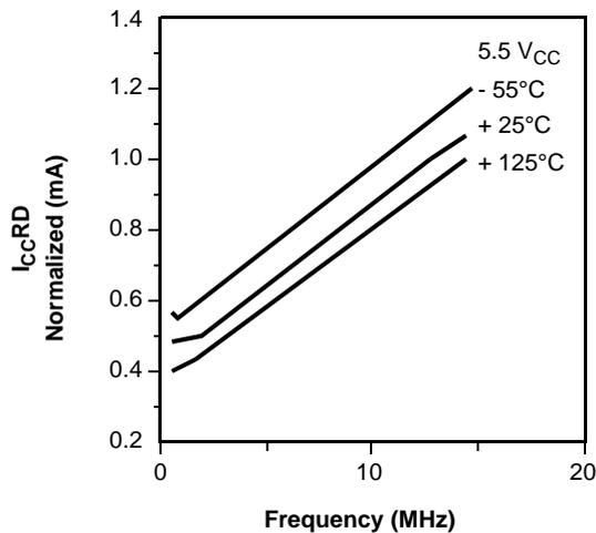
Normalized  $I_{CC}(\text{RD})$  @ 25% Over the  $V_{CC}$  Range and Frequency
