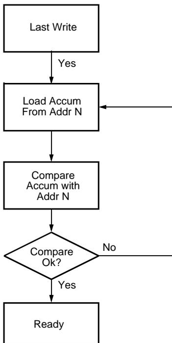
The Toggle Bit can eliminate the chore of saving and fetching the last address and data in order to implement DATA Polling. This can be especially helpful in an array comprised of multiple X28HC64 memories that is frequently updated. Toggle Bit Polling can also provide a method for status checking in multiprocessor applications. The timing diagram in Figure 4 illustrates the sequence of events on the bus. The software flow diagram in Figure 5 illustrates a method for polling the Toggle Bit.
