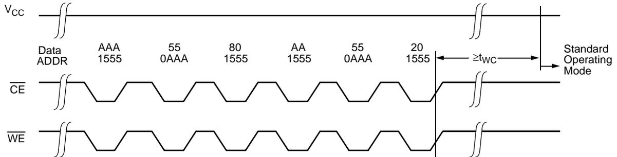
Figure 9. Software Sequence to Deactivate Software Data Protection
