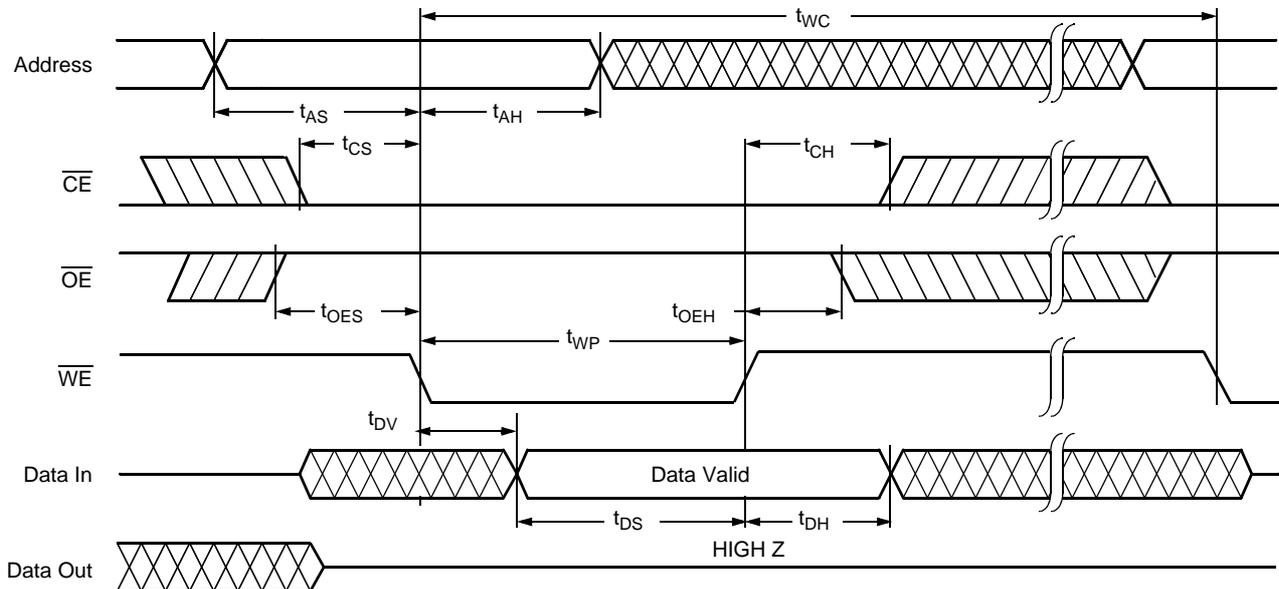
Notes: (5)  $t_{WC}$  is the minimum cycle time to be allowed from the system perspective unless polling techniques are used. It is the maximum time the device requires to automatically complete the internal write operation.
