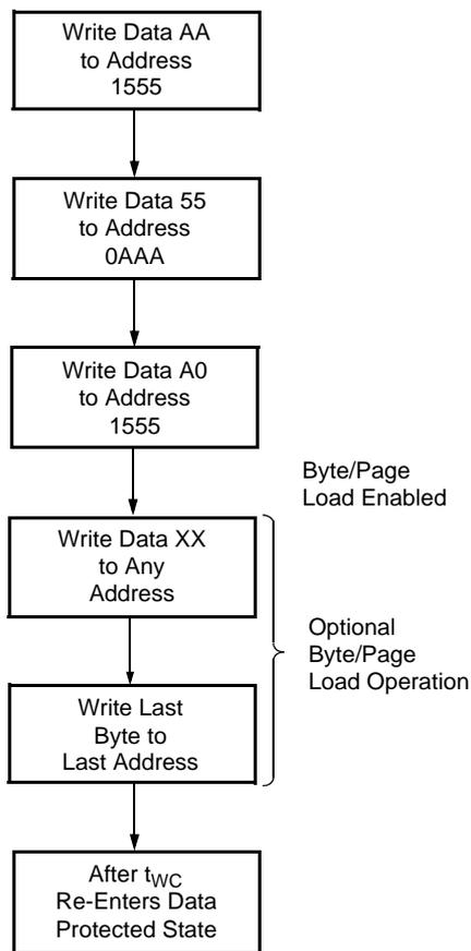
Regardless of whether the device has previously been protected or not, once the software data protection algorithm is used, the X28HC64 will automatically disable further writes unless another command is issued to deactivate it. If no further commands are issued the X28HC64 will be write protected during power-down and after any subsequent power-up.
