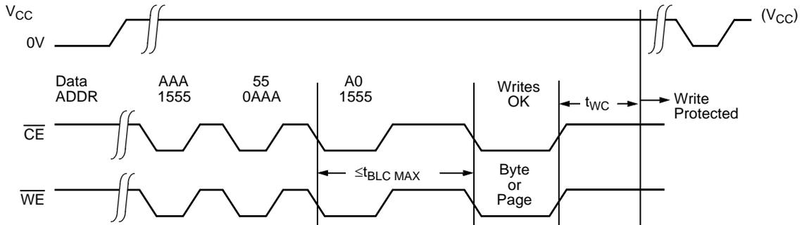
Figure 7. Write Sequence for Software Data Protection
