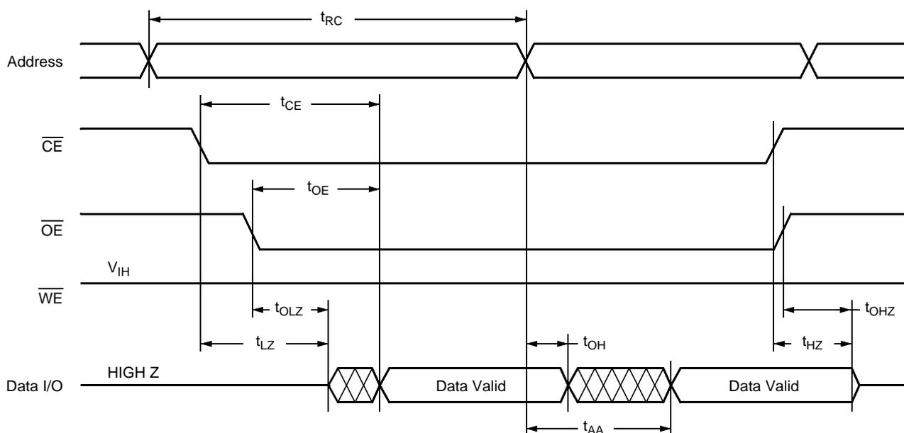
Note: (4)  $t_{LZ}$  min.,  $t_{HZ}$ ,  $t_{OLZ}$  min., and  $t_{OHZ}$  are periodically sampled and not 100% tested.  $t_{HZ}$  max. and  $t_{OHZ}$  max. are measured from the point when  $\overline{CE}$  or  $\overline{OE}$  return HIGH (whichever occurs first) to the time when the outputs are no longer driven.
