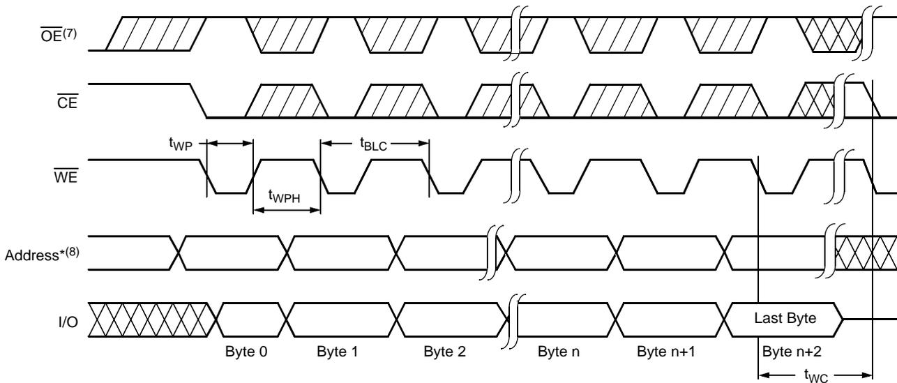
\*For each successive write within the page write operation,  $A_6$ - $A_{12}$  should be the same or writes to an unknown address could occur.
