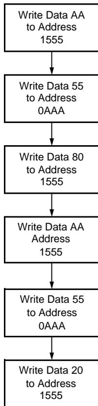
In the event the user wants to deactivate the software data protection feature for testing or reprogramming in an EEPROM programmer, the following six step algorithm will reset the internal protection circuit. After  $t_{WC}$ , the X28HC64 will be in standard operating mode.
