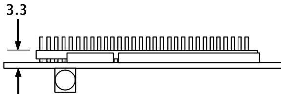
Figure 10.1-1 Thickness of module variant without SIM holder
