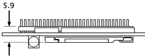
Figure 10.1-2 Thickness of module variant with SIM holder
