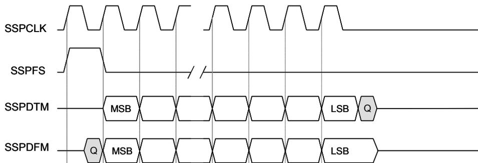
Figure 5.10-2 PCM Frame format for a single transfer
