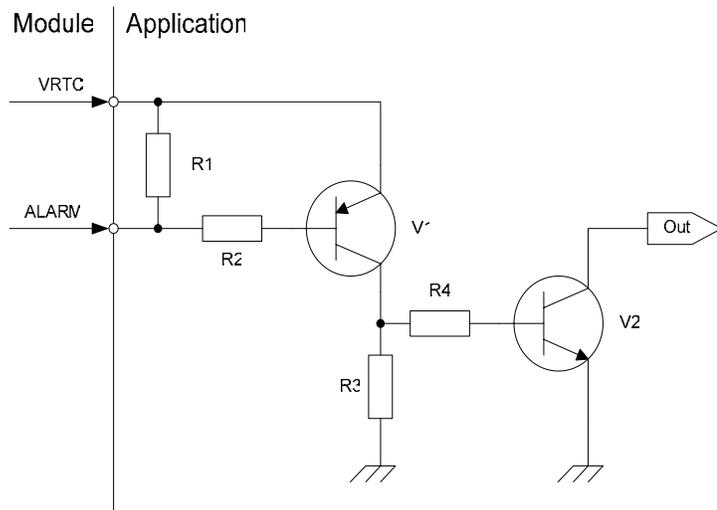
Figure 5.20-2 Typical host-side circuit for ALARM output
