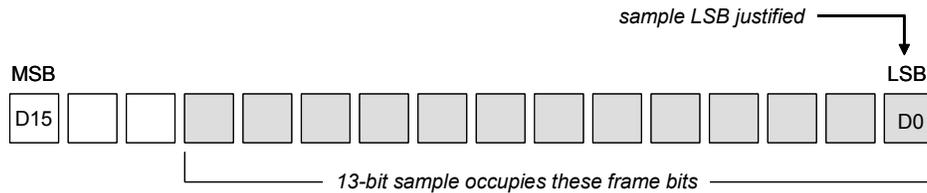
Figure 5.10-1 Typical 16-bit PCM Voice Sample Word Format
