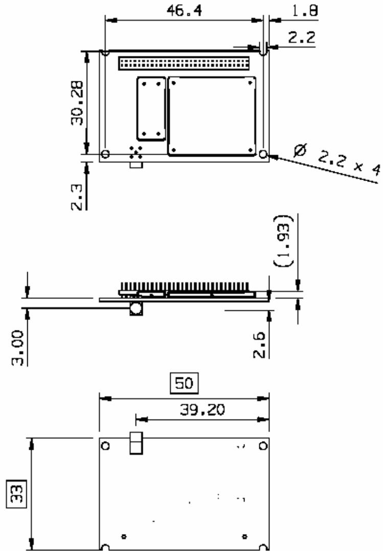
Figure 4.2-2 Dimensions of the Wireless modem (Legacy variant)
