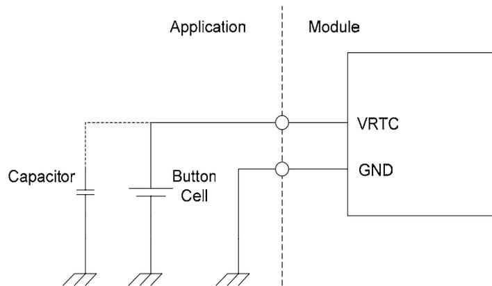
Figure 5.20-1 VRTC connection
