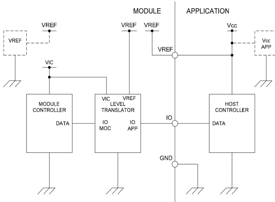
Figure 5.6-1 Level shifter arrangement
