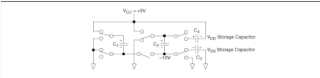
Figure 14. Charge Pump — Phase 3 -  $V_{SS}$  Charge Transfer
