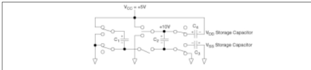
Figure 16. Charge Pump — Phase 1 -  $V_{DD}$  Charge Transfer
