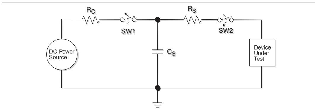
Figure 18. ESD Test Circuit for Human Body Model
