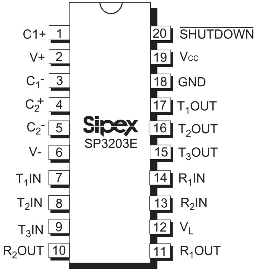
Figure 7. SP3203E Pinout Configuration
