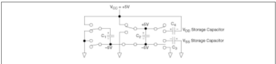
Figure 15. Charge Pump — Phase 2 -  $V_{DD}$  Charge Storage
