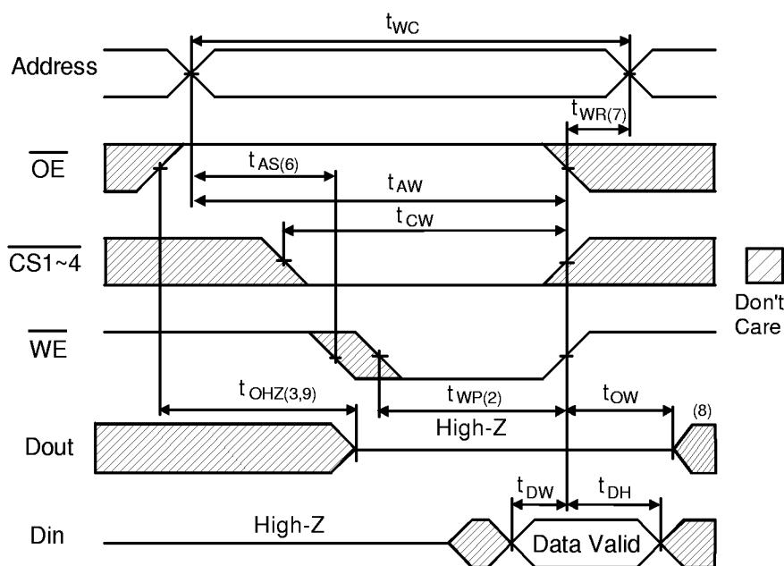
**Write Cycle No.2 Timing Waveform<sup>(1,9)</sup>**
