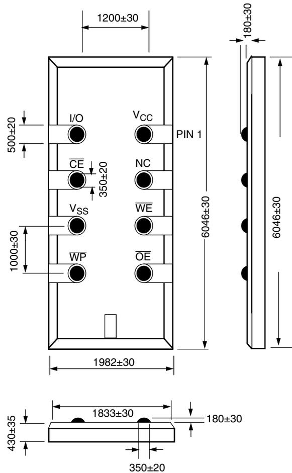
**NOTE: ALL DIMENSIONS IN  $\mu\text{M}$  (to convert into inches,  $1\mu\text{m} = 3.94 \times 10^{-5}$  inch)
