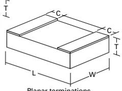
Alternative styles for surface mounting resistors
