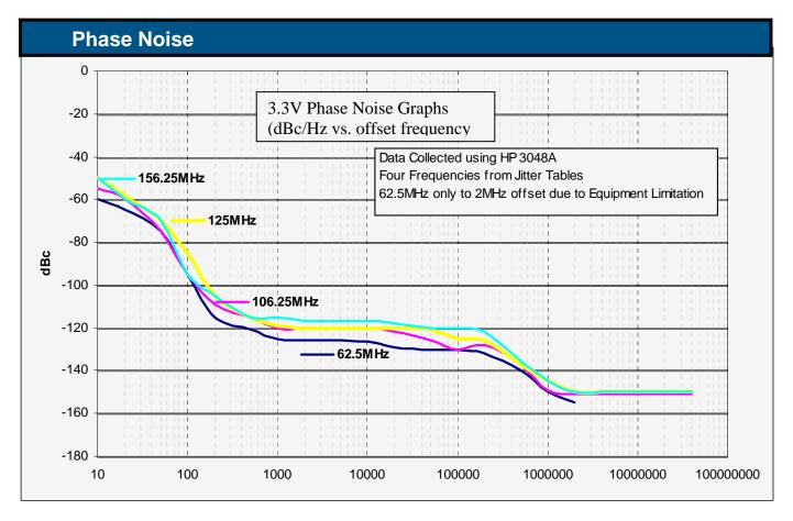
Jitter is frequency dependent. Below are typical values at select frequencies.
