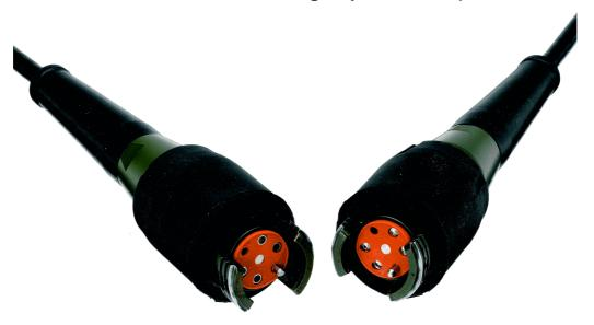
This environmental legacy hermaphroditic fibre optic lens connector facilitates the inter-connection of multiple identical fibre optic cable assemblies known as daisy chaining, thus eliminating the need for polarising the assemblies and the use of in-line adapters. The Connector is available in 1 to 4 way configurations for a variety of multi-mode, single mode fibres and both 850 and 1300nm applications and is inter-mateable/interchangeable with other manufacturers equivalent products.
