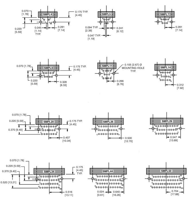
SUGGEST 0.105 [2.66] Ø HOLES IN PRINTED BOARD FOR CONNECTOR MOUNTING HOLES
