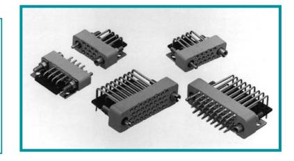
SMPL Series connectors are high reliability, high density, rectangular connectors meeting the performance requirements of MIL-DTL-28748. Termination style is right angle printed board mount. SMPL Series connectors are intermateable with Positronic SGM and SGMC series connectors.
