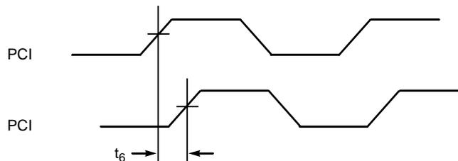
**CPU Clock Cycle-Cycle Jitter**
