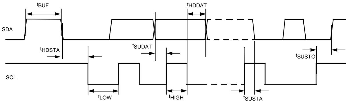
Figure 2. M\_BUS TIMING
