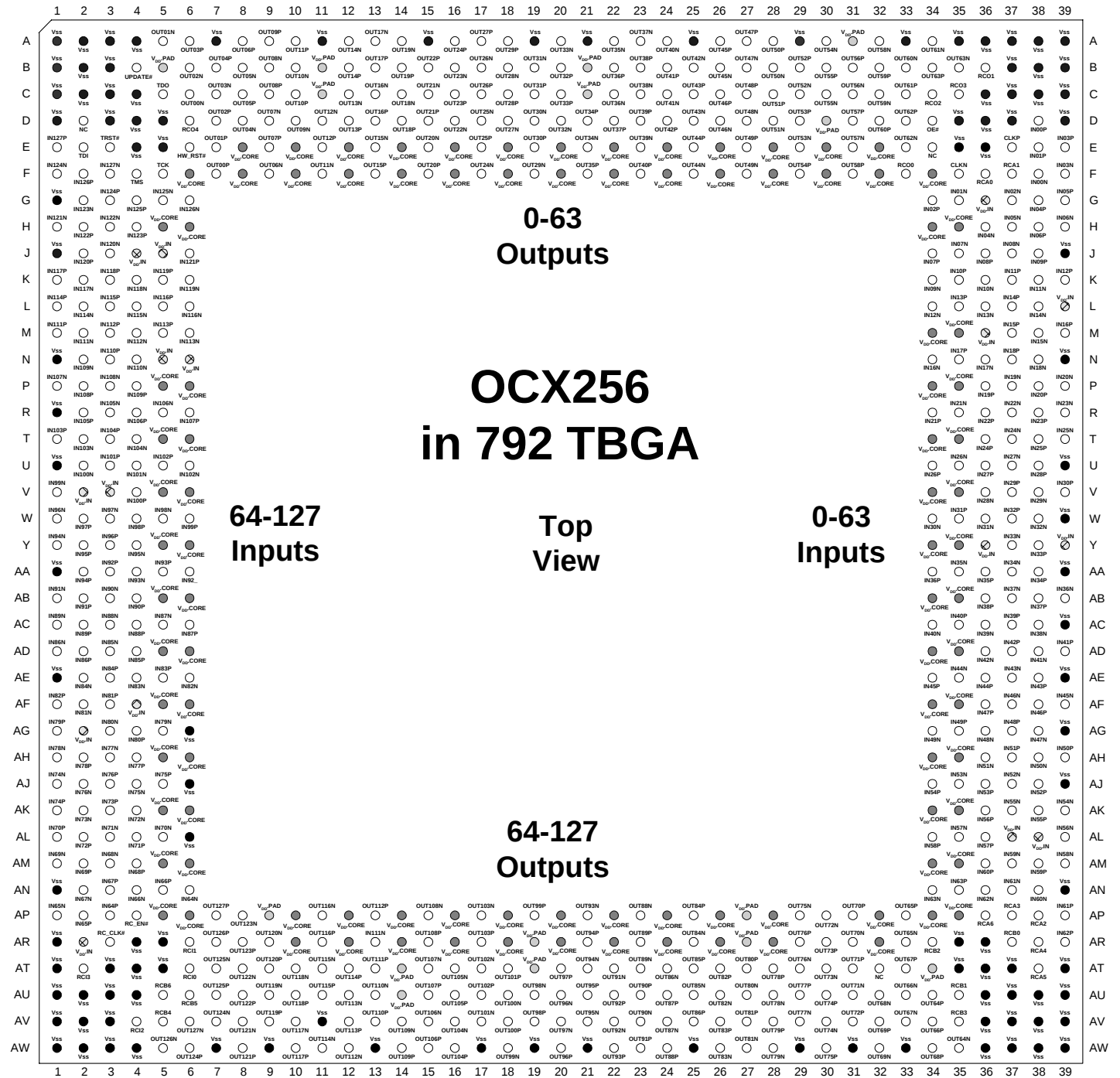
Figure 18 OCX256 Package Pinout
