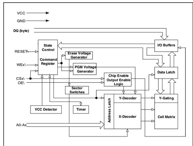
A system reset would then also reset the FLASH device, enabling the system microprocessor to read the boot-up firmware from the FLASH memory array. The device offers two power-saving features. When addresses have been stable for a specified amount of time, the device enters the AUTOMATIC SLEEP MODE. The system can also place the device into the STANDBY mode. Power consumption is greatly reduced in both these modes.
