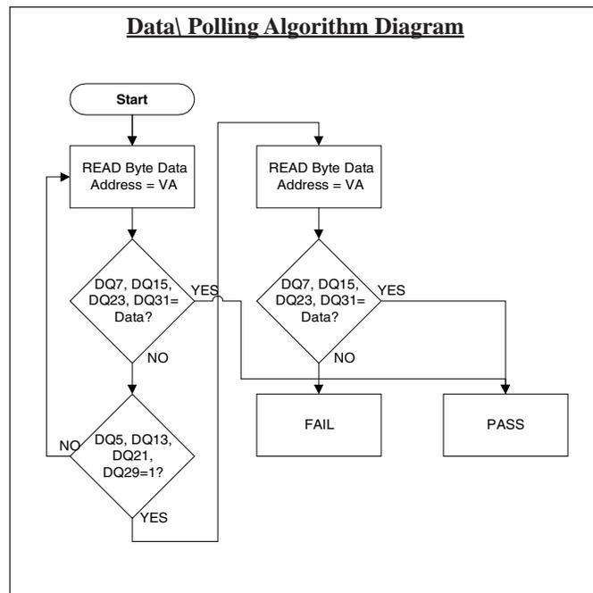
Algorithm is complete, the device outputs the datum PROGRAMMED into each of these status bits. The system must provide the PROGRAM address to READ valid status information. If a PROGRAM address fails within a protected sector, Data\ Polling is active for approximately 1uS, then the device returns to reading array data.
