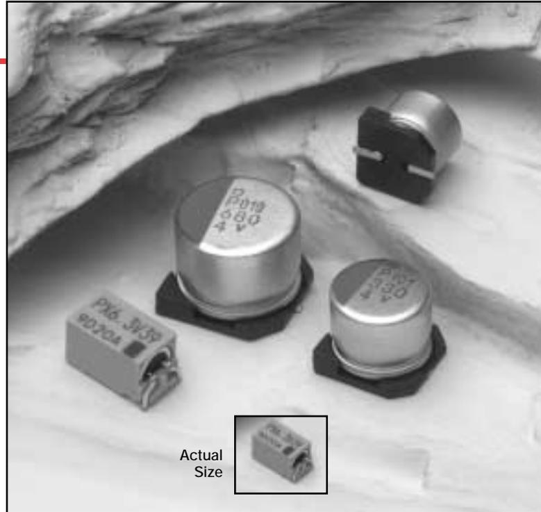
The PX series is a new surface mount capacitor series that uses a polymer as the electrolyte. This allows for very low impedance and for extended useful lifetimes. Available in vertical and horizontal case styles, the PX series is designed for use in DC-DC converters and voltage regulators or any other application where a low impedance cap is required. The PX series capacitors can also be used as a surface mount option for an OS-CON™ capacitor.
