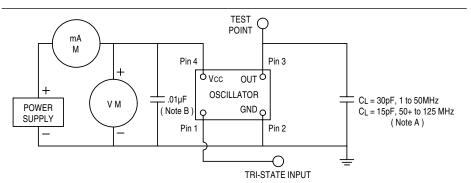
NOTE: A. CL includes probe and fixture capacitance. NOTE: B. An external .01µF bypass capacitor close to package ground and VCC pin is required
