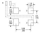
\*External high frequency power supply decoupling required. Scale: None ( Dimensions in  $\frac{mm}{inches}$  )
