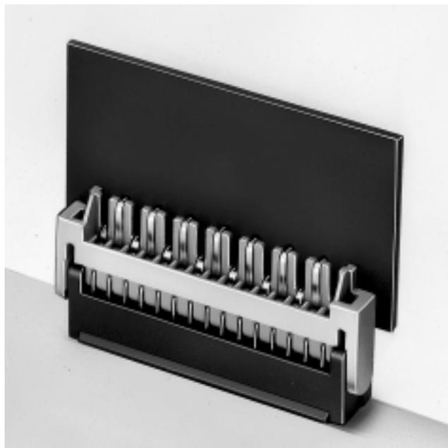
**Hinge type board to board connectors which allow mated PCB's to move 90° in respect to one another while electricity is turned on. The hinge compensates for slight misalignments between circuit boards to assure a secure connection even if the boards are laterally out of line.**
