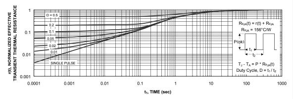
Figure 11. Transient Thermal Response Curve.
