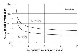
Figure 4. On-Resistance Variation with Gate-to-Source Voltage.
