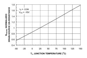
Figure 3. On-Resistance Variation with Temperature.
