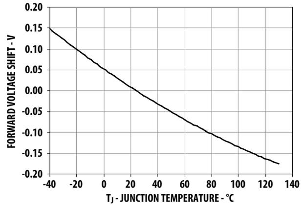
Figure 8. Relative Forward Voltage vs Junction Temperature
