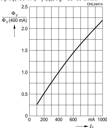
Relativer Lichtstrom<sup>2)</sup> Seite 20Relative Luminous Flux<sup>2)</sup> page 20 $\Phi_V/\Phi_V(400 \text{ mA}) = f(I_F); T_S = 25^\circ\text{C}; \text{ yellow}$
