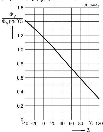
Relativer Lichtstrom<sup>2)</sup> Seite 20Relative Luminous Flux<sup>2)</sup> page 20 $\Phi_V/\Phi_{V(25^\circ\text{C})} = f(T_j); I_F = 400 \text{ mA}; \text{yellow}$
