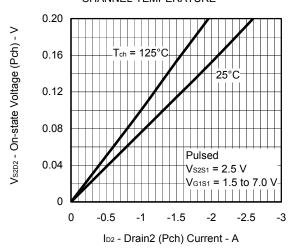
ON-STATE RESISTANCE (Pch) vs. CHANNEL TEMPERATURE
