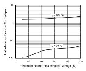
Fig. 3 - Typical Reverse Characteristics
