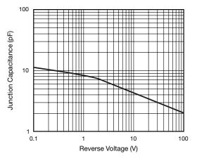
Fig. 4 - Typical Junction Capacitance
