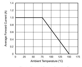
Fig. 1 - Forward Current Derating Curve
