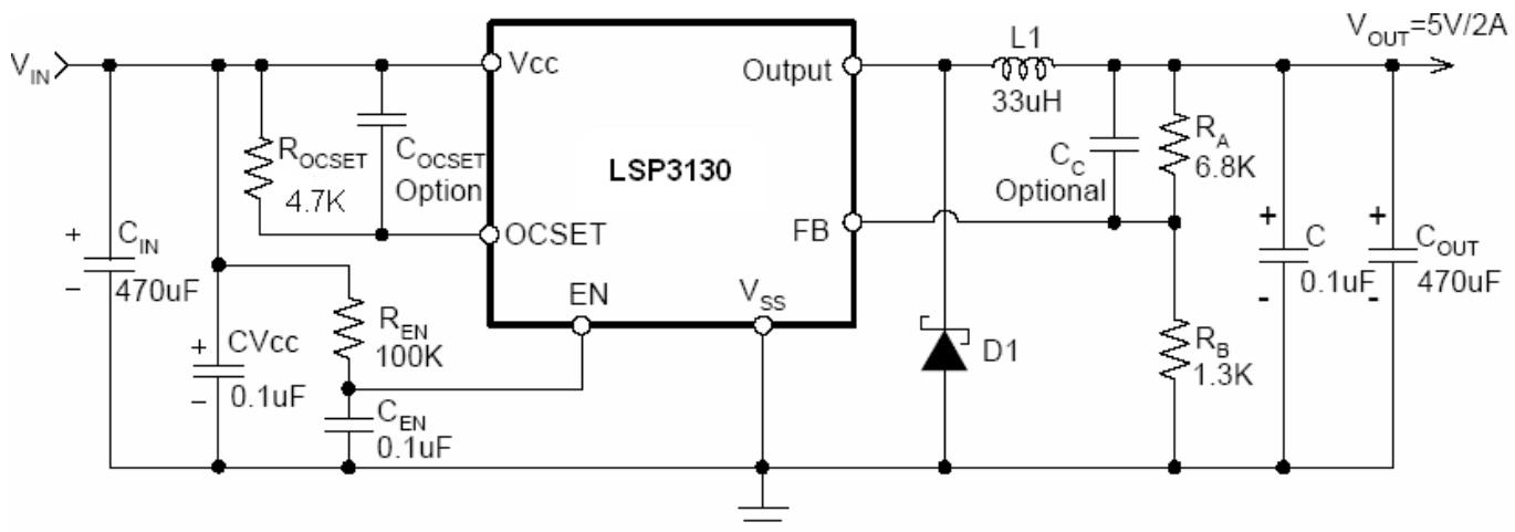
Note1:C<sub>IN</sub>/C<sub>OUT</sub> can be Electro capacitor or Tan capacitor; The typical C<sub>IN</sub> Electro capacitor is 470uF/35V, the typical C<sub>IN</sub> Tan capacitor is 100uF/35V; The typical C<sub>OUT</sub> Electro capacitor is 470uF/16V, the typical C<sub>OUT</sub> Tan capacitor is 22uF/16V;
