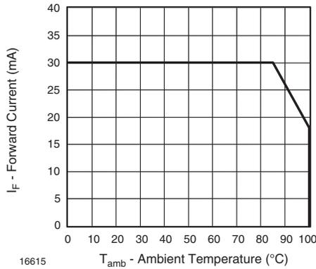
Figure 1. Max. Permissible Forward Current vs. Ambient Temperature
