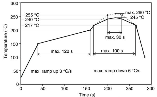
Figure 12. Vishay Lead (Pb)-free Reflow Soldering Profile (acc. to J-STD-020)
