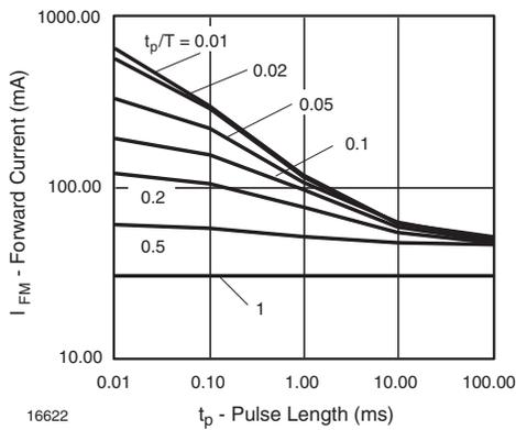
Figure 2. Permissible Forward Current vs. Pulse Length
