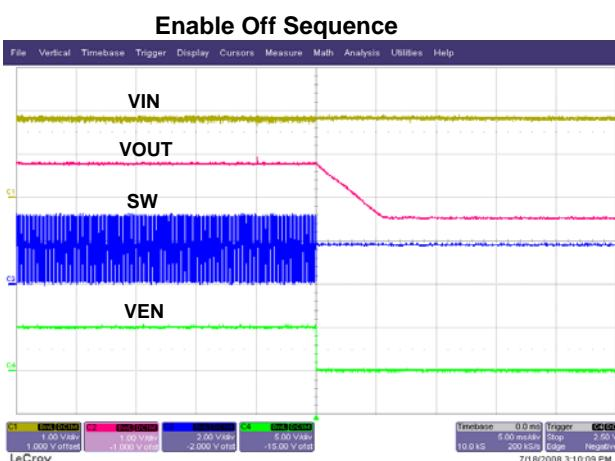
V<sub>IN</sub>=1.8V, V<sub>OUT</sub>=2.8V, I<sub>OUT</sub>=10mA, EN=5 to 0V
