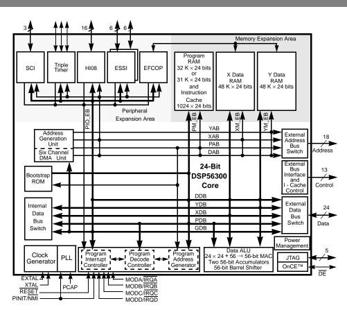
Figure 1. DSP56311 Block Diagram
