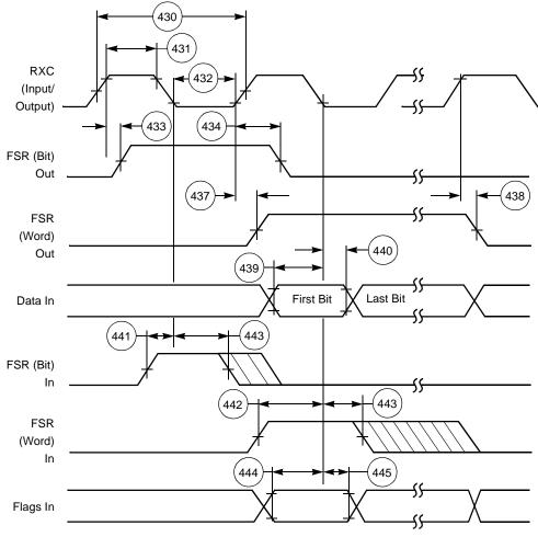
Figure 2-32. ESSI Receiver Timing
