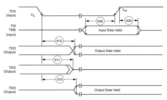
Figure 2-37. Test Access Port Timing Diagram
