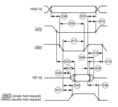
Figure 2-22. Read Timing Diagram, Non-Multiplexed Bus, Double Data Strobe
