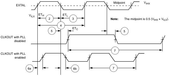
Figure 2-2. External Clock Timing
