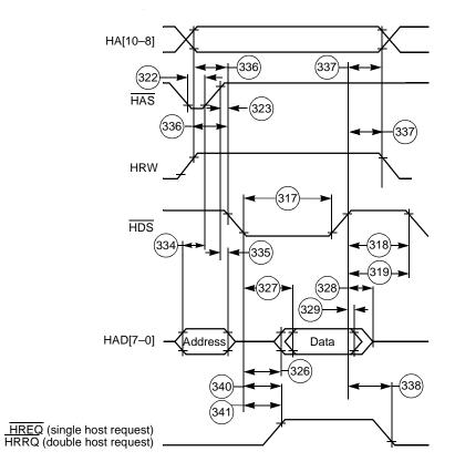
Figure 2-25. Read Timing Diagram, Multiplexed Bus, Single Data Strobe
