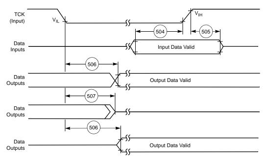
Figure 2-36. Boundary Scan (JTAG) Timing Diagram
