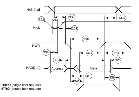
Figure 2-28. Write Timing Diagram, Multiplexed Bus, Double Data Strobe
