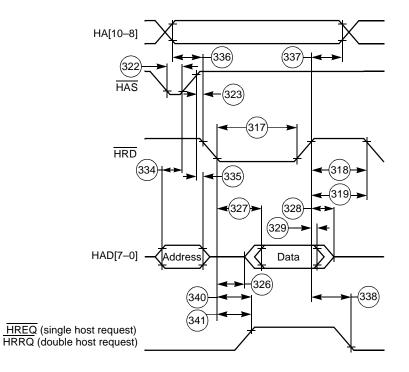
Figure 2-26. Read Timing Diagram, Multiplexed Bus, Double Data Strobe
