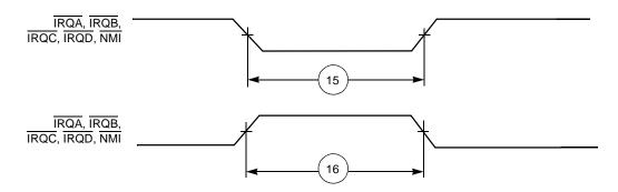
Figure 2-5. External Interrupt Timing (Negative Edge-Triggered)
