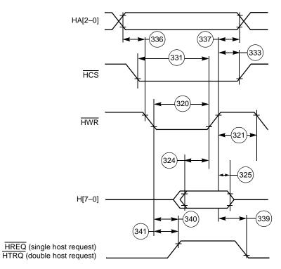
Figure 2-24. Write Timing Diagram, Non-Multiplexed Bus, Double Data Strobe
