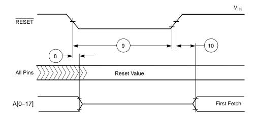
Figure 2-3. Reset Timing
