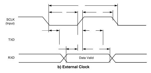
Figure 2-29. SCI Synchronous Mode Timing
