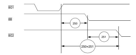
Figure 2-19. Asynchronous Bus Arbitration Timing
