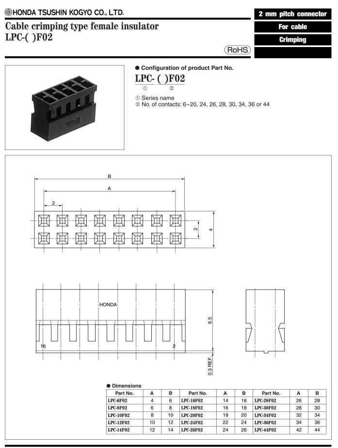
Mating connectors: LPC series cable crimping type female contacts
