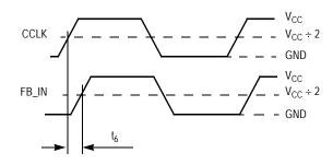
Figure 2. Static Phase Offset Test Reference
