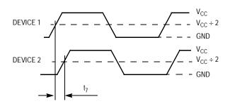
Figure 4. Device-to-Device Skew
