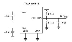
Test Circuit for t<sub>8</sub>, Output slew rate on –1H, –5 device
