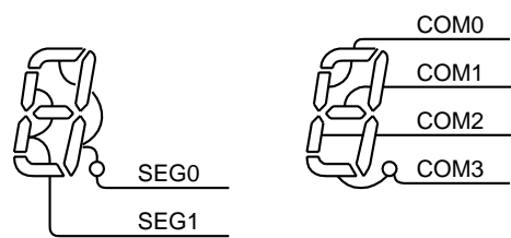
Figure 13-6 Example of COM, SEG Pin Connection (1/4 Duty)
