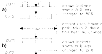
Fig. 7 Effect of Changing the Duty Cycle during a PWM Cycle
