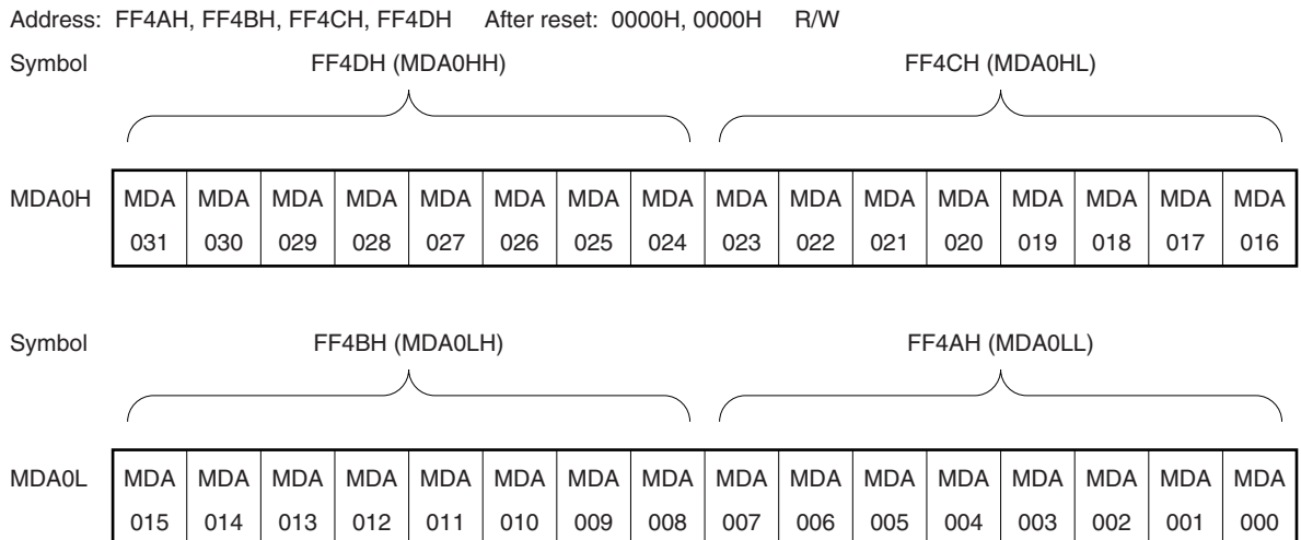
Figure 20-3. Format of Multiplication/Division Data Register A0 (MDA0H, MDA0L)
