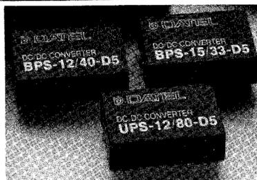
All models include internal Pi-type filters to minimize reflected ripple current. Other features include continuous short-circuit protection with automatic restart, 300V dc isolation, and no derating over the full operating temperature range of -25 to +71 °C.
