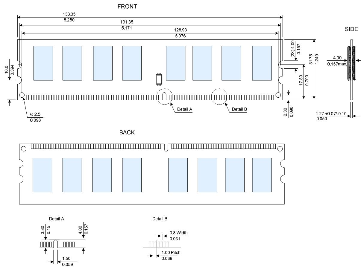
Note: All dimensions are typical with tolerances of  $\pm 0.15$  (0.006) unless otherwise stated.
