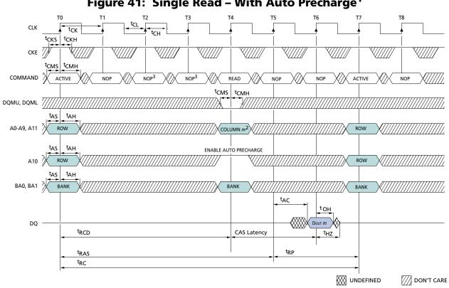
Figure 41: Single Read – With Auto Precharge<sup>1</sup>
