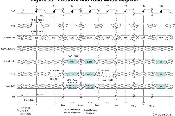
Figure 33: Initialize and Load Mode Register<sup>1,2</sup>
