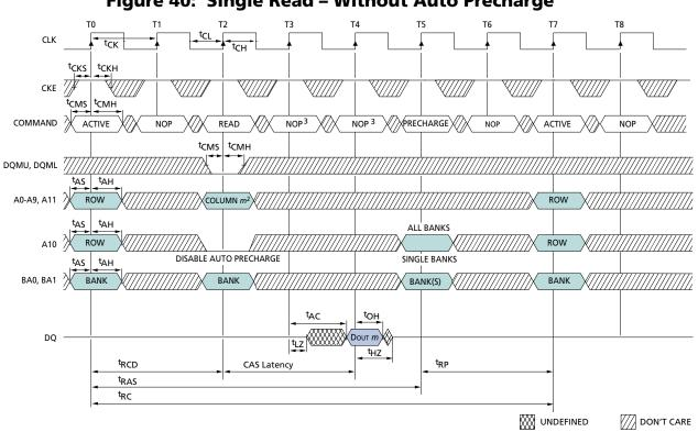
Figure 40: Single Read – Without Auto Precharge<sup>1</sup>
