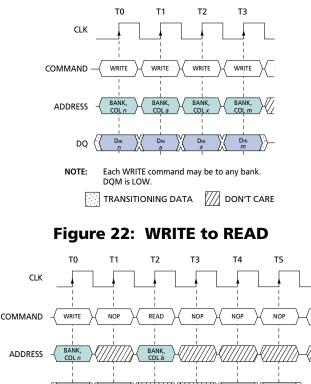
The WRITE command may be to any bank and the READ command may be to any bank. DOM is LOW. CAS latency = 2 for illustration. TRANSITIONING DATA
