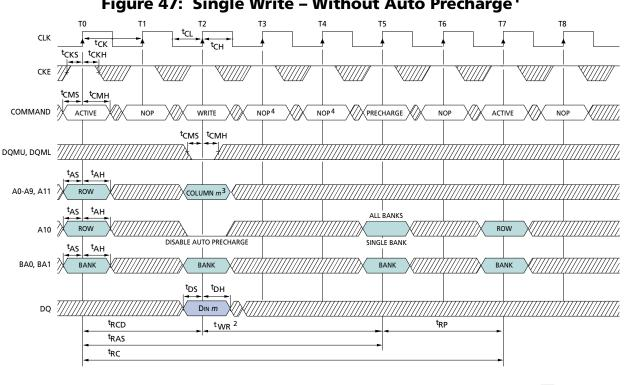
Figure 47: Single Write – Without Auto Precharge<sup>1</sup>
