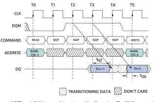
NOTE: A CAS latency of three is used for illustration. The READ command may be to any bank, and the WRITE command may be to any bank.
