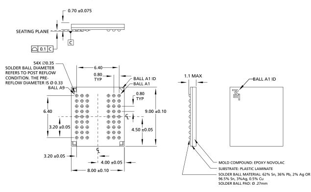
Figure 52: 54-Ball FBGA (8mm x 9mm)
