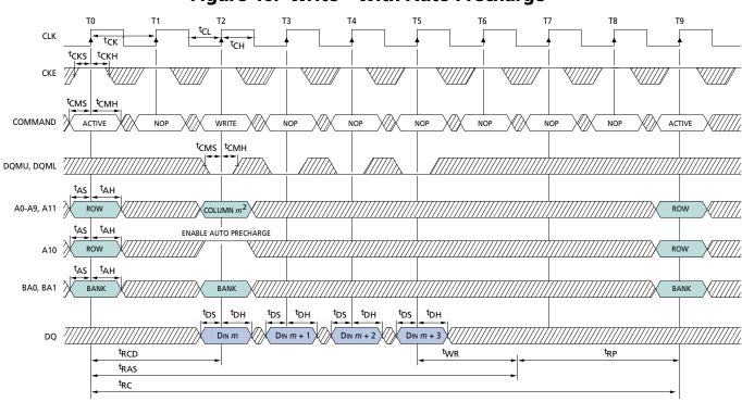
Figure 46: Write – With Auto Precharge<sup>1</sup>
